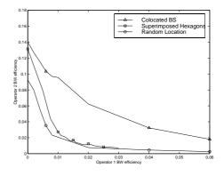
Figure 4 – The figure shows the bandwidth efficiency for various base station locations and 5% outage. Processing gain is 100.
