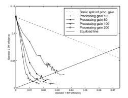
Figure 3 – Spectrum sharing using DS-CDMA. The figure shows the bandwidth efficiency for different processing gains. The cell layout is superimposed hexagons.
