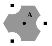
Figure 2 – The area (A) that is supported by the circular basestation in the middle. The squares represent interfering basestations.
